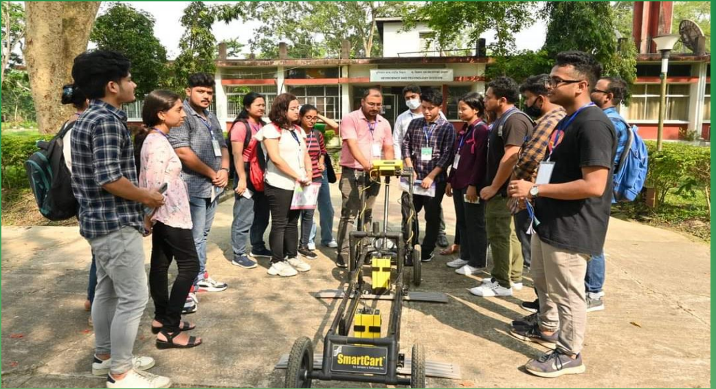
Fig (52): Mr. Sausthov M. Bhattacharyya, Sr. Technical Officer of Geoscience & Technology Division , CSIR-NEIST is seen demonstrating working principles and use of GPR (Ground Penetrating Radar) to the participants of GeoIBR'22 (7 th June 2022).
